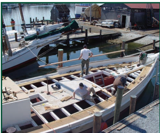
Skipjack restoration work on the Lady Katie. Photograph courtesy of the Chesapeake Bay Maritime Museum.
